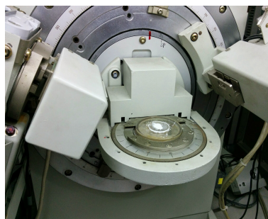
Figure 5.4: Experimental setup for measuring an XRD pattern
