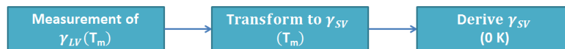
Figure 2.5: Summary of the process to obtain the surface free energy at 0K.
