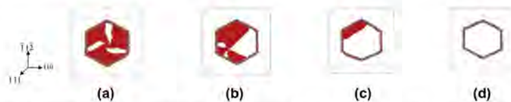
Fig. 3. Modeling of the interstitial Frank loop of diameter d = 12.1 nm with the sides oriented along \langle 112 \rangle directions at T = 300 K at the times (a) 1 ps, (b) 9 ps, (c) 12 ps and (d) 15 ps. The orientation of the crystal is the same in all figures.
