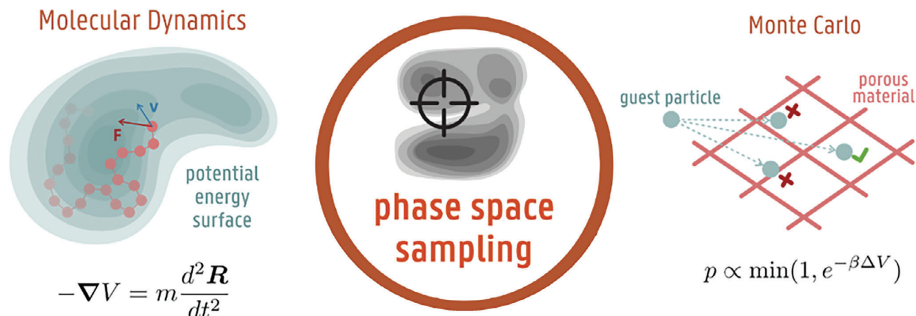
Figure 10. Illustration of dynamics phase space sampling methods. Molecular dynamics propagates the system through time by integrating Newton's equations of motion (left). Monte Carlo methods are based on accepting random insertion/deletion moves through importance sampling. Reproduced with permission. [121] Copyright 2024, Royal Society Publishing.
