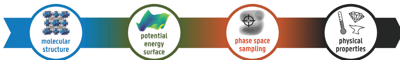
Figure 3. The sequence of a molecular modeling exercise, from left to right: building a structural model, modeling the potential energy surface, phase space sampling, and deriving target physical properties. Reproduced with permission. [58] Copyright 2023, Royal Society Publishing.
