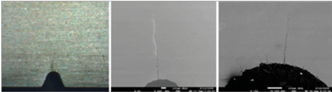
Figure 9: Some examples of crack appearance during the constant load testing.
