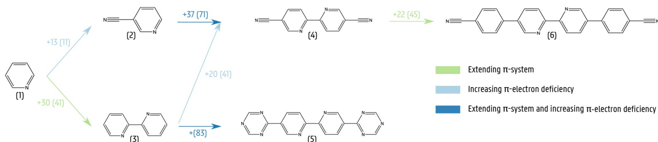
Figure 4. Influence of extending the \pi -system and increasing the \pi -electron deficiency of the linkers on the position of the main absorption peak. Shifts are given in nm. We report experimental results along with the computational findings between parentheses. The computational results are obtained at the B3LYP/6-31 + + G** level of theory with acetonitrile as solvent and are discussed in Sections 3.2 and 3.4.
