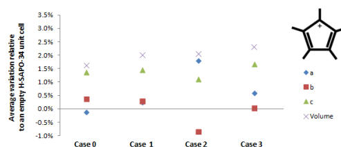
Figure 7: Average variation of unit cell parameters and volume relative to an empty H-SAPO-34 unit cell at 623 K and 1 atm of PMCP + for a 50 ps MD simulation.
