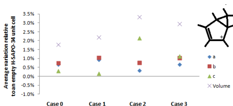
Figure 4.5: Average variation of unit cell parameters and volume relative to an empty H-SAPO-34 unit cell at 623 K and 1 atm of 5-3-CP + for a 50 ps MD simulation.
