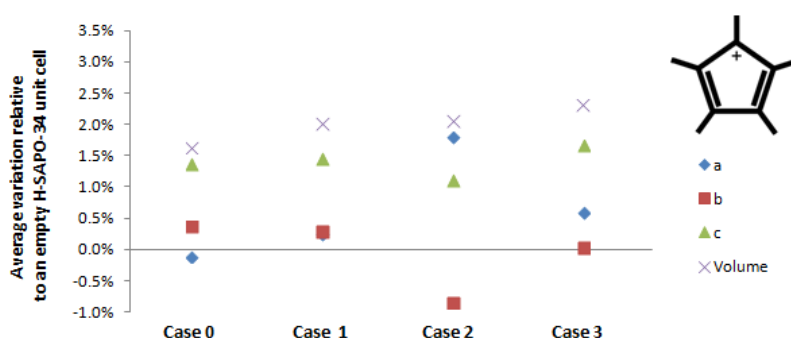
Figure 4.6: Average variation of unit cell parameters and volume relative to an empty H-SAPO-34 unit cell at 623 K and 1 atm of PMCP + for a 50 ps MD simulation.
