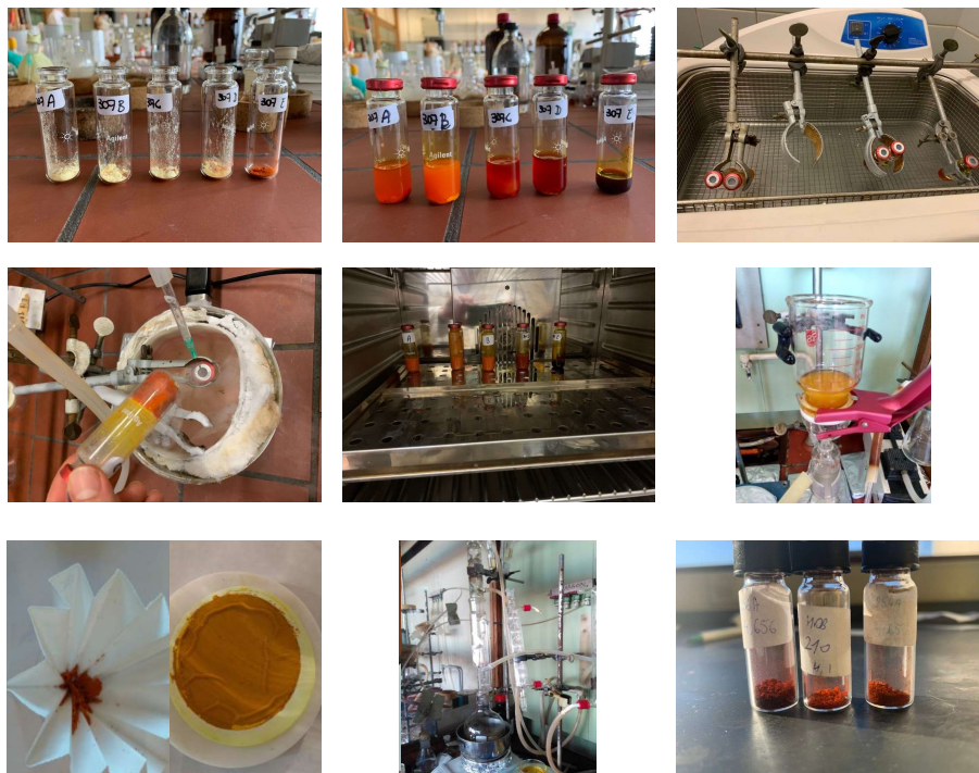
Figure 4: Visual representation of the workflow to synthesize COFs. In the first picture the solid reagents are added to the vials, after which the solvents and the acid catalysts are added and the vials are capped (picture 2). Then the vials were sonicated (picture 3) after which they are repeatedly frozen in liquid nitrogen and pumped to remove all traces of oxygen from the reaction (picture 4). Finally, they are placed in a pre-heated oven at a set temperature for a pre-determined time (typically 120 °C, 72 h, picture 5). The vials are then opened, filtered over a membrane filter, and washed with a range of solvents (picture 6). The materials are then placed in a paper filter to use for Soxhlet extraction (picture 7 and 8). After Soxhlet extraction and drying under vacuum the COFs are stored in vials at room temperature (picture 9).
