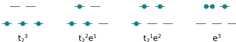
Figure 3.11: Schematic representation of a possible micro-state for the electron configurations in octahedral d^3 complexes.
