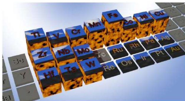
Figure 6.1: Visualization of the earth abundance and relative production of CO 2 for the TMs. The height of the pillar for each metal indicates its crustal abundance on a log scale. The black bar on each metal shows, also on a log scale, the relative amount of CO 2 produced through mining and purification for each metal. 240 Tc is shown but is radioactive and unstable. From Ref. 239 . Reprinted with permission from AAAS.
