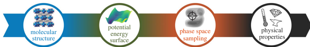
Figure 2. The sequence of a modelling exercise where one starts from a realistic atomic level representation for the material, determines the multidimensional potential energy surface (PES). This PES needs to be sampled in the interesting regions after which the target properties can be derived. (Online version in colour.)
